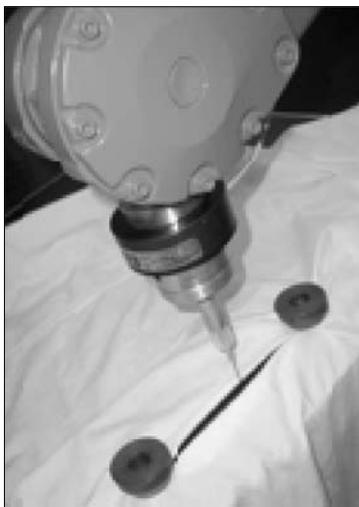
Figure 2: Using an industrial robot attached to a six-axis force sensor to measure the haptic properties of neoprene. Neoprene was chosen for initial testing as it was found to have similar haptic properties to bovine liver. Differing gauges of needle were tested with a diverse array of tip geometries. These results have been stored in a material library for future reference and input into our needle model.
